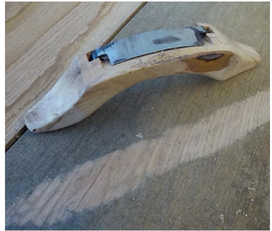
19 Shave made for the production of the replica door. Photo Peter Massey
