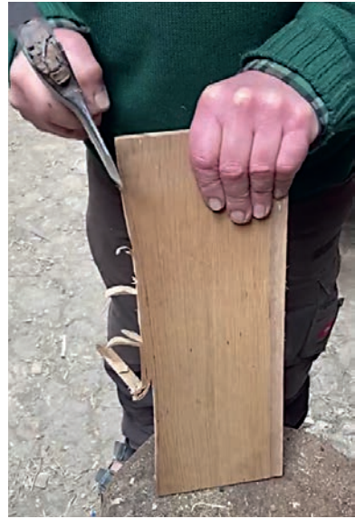
28 Waste is removed with a side axe. Photo E. Massey
