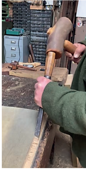
21 (far left) Setting out the rebates. Photo E. Massey
