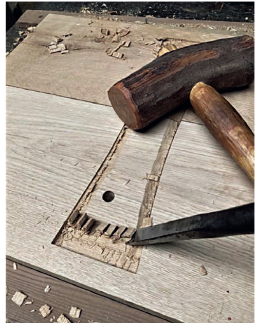
32 Cutting out the housing with a chisel. Photo E. Massey
