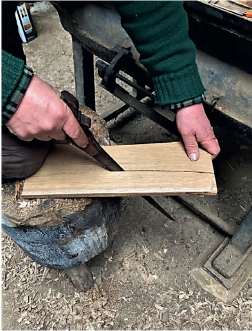
29 Cutting out the waste using a saw. Photo E. Massey
