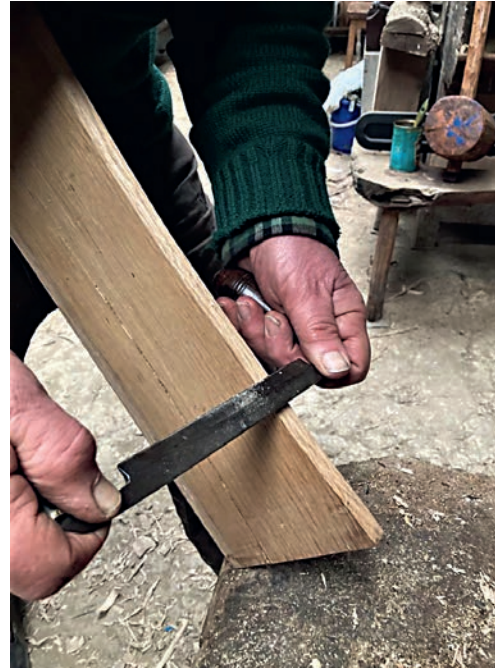
30 Truing up the edges with a draw knife. Photo E. Massey
